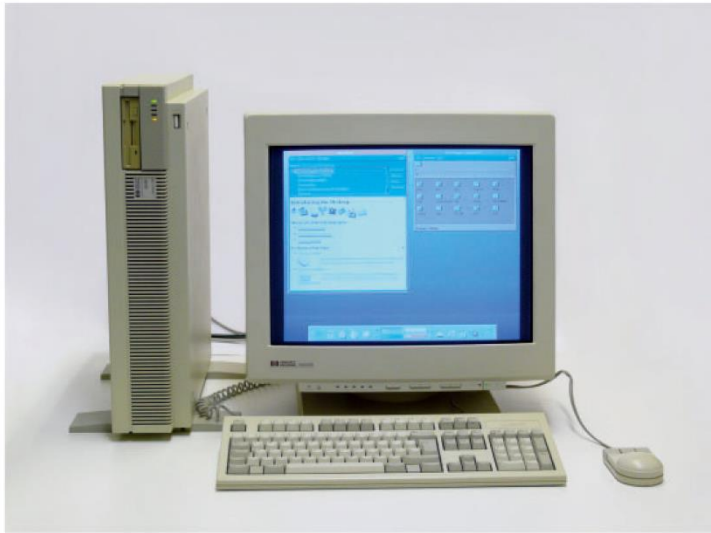
HP-9000 desktop workstation running the Unix-based system HP-UX. Image: Thomas Schanz//CC-BY-SA 3.0.
